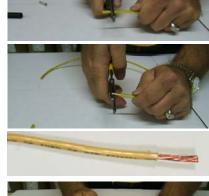
Step 2: Crimp connection. Insert stripped wires from one end of the Tuff Cable into number 10 butt splice connector provided in splice kit and crimp the connection well. Repeat this procedure for the other end of the Tuff Cable.
