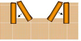
Step 5. Cut 1" of both ends of subsequent Splice Plate piece(s) so it covers the ZMesh edge to be repaired, plus the ends of the other Splice Plate pieces.
