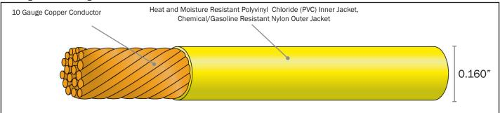
Conductor10 Gauge CopperInner JacketHeat and Moisture Resistant Polyvinyl Chloride (PVC)Outer JacketNylon (Polyamide)Minimum Spacing2 "Operating Voltage65 VAC or LessMaximum Temperature194°F (90°C)Output WattageUp to 11 watts per footWarranty25 Year Limited WarrantyListing AgencyETL (Intertek Testing Laboratory)
