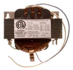
All single Heatizon Systems Transformers require one pair of Cold Leads (SLC 500 systems require one pair of Cold Leads for the beginning and ending points of the Tuff Cable or ZMesh heating element). One of the Cold Leads from any given pair connect to the common tap located at the back of the Transformer and the other Cold Lead connects to one of the voltage taps at the front of the transformer.
