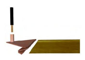
**Step 1: Connect Cold Lead to Transition Plate.** Connect the transition plate to Cold Lead by stripping back 1 inch of insulation from the Cold Lead. Insert the exposed Cold Lead into the butt splice connector on transition plate and crimp twice.
