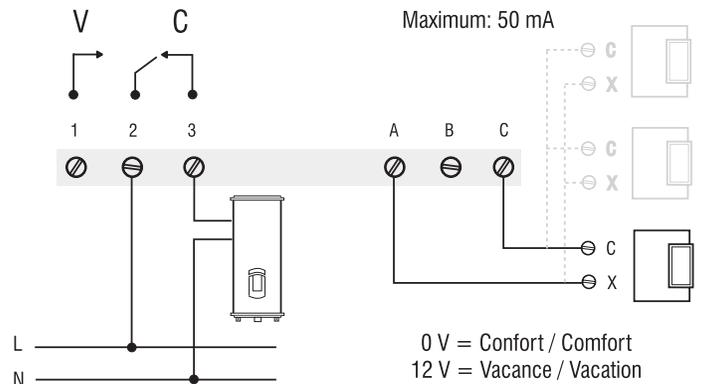
Figure 5: Dry contact to thermostat
