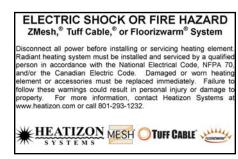
It is not recommend that you ever remove any of the covers on the Control Unit. Never open your Heatizon Systems Control Unit without first turning the power to the Control Unit completely off by turning both the Control Unit Switch, if so equipped, and the Circuit Breaker in the Electric Distribution Panel to the off position.
