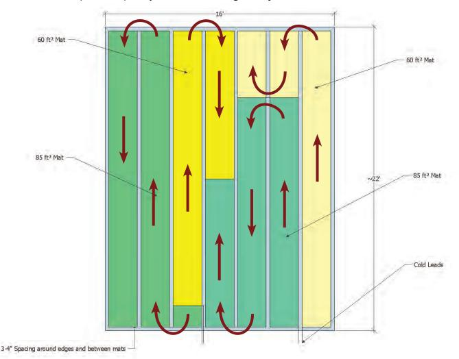
Using the SnowMeltz 290 kit (SM-50W277-37W240-290) to fill a space that is approximately 330 square feet, with 3 inch spacing around the perimeter and between mats. This example has no control joints, therefore no jumpers would be used. All the cold leads would meet the incoming power at the activator device (M326ARS-2Z), where all the electrical connections would be made.
